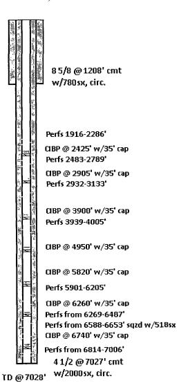
Circ cmt from 60' to surface 25sx plug from 1158-1258' 85/8 @1208' cmt w/780sx, circ. 25sx plug from 1730-1830' CIBP @ 1875' w/35' cap Perfs 1916-2286' CIBP @ 2425' w/35' cap Perfs 2483-2789' CIBP @ 2905' w/35' cap Perfs 2932-3133' CIBP @ 3900' w/35' cap Perfs 3939-4005' CIBP @ 4950' w/35' cap CIBP @ 5820' w/35' cap Perfs 5901-6205' CIBP @ 6260' w/35' cap Perfs from 6269-6487' Perfs from 6588-6653' sgzd w/518sx CIBP @ 6740' w/35' cap Perfs from 6814-7006' 41/2@7027'cmt TD @7028' W/2000sx, circ.
