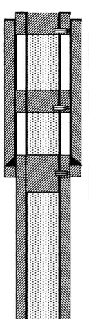
5. PUH & perf @ 250' & sqz 80 sx Class "C" cmt from 250' to surf, CIRC all strings to surf. (Water Board)
