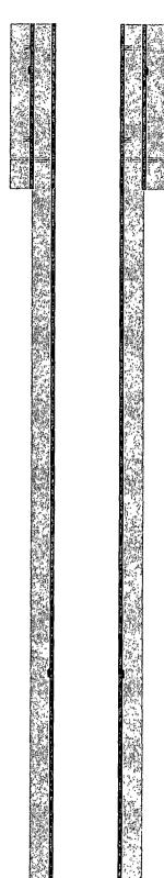
14-3/4" hole @ 1615' 9-5/8" csg @ 1615' DVT @ 600' w/ 955sx-TOC-Surf-Circ
