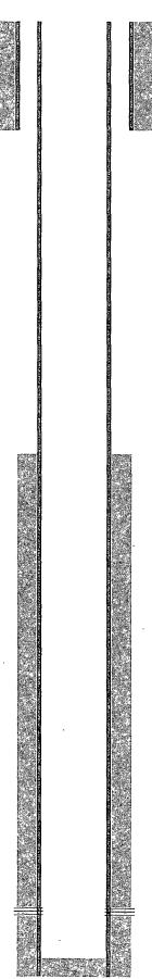
12-1/4" hole @ 621' 8-5/8" csg @ 621' w/ 1105sx-TOC-Surf-Circ
