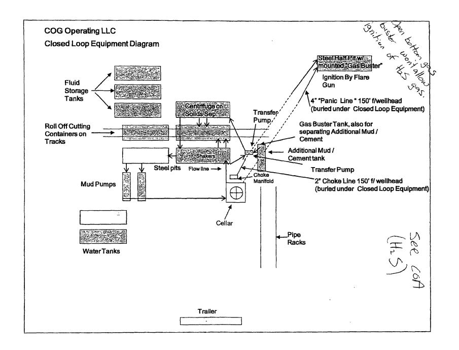
All drilling fluid circulated over shaker(s) with cuttings discharged into roll off container.
