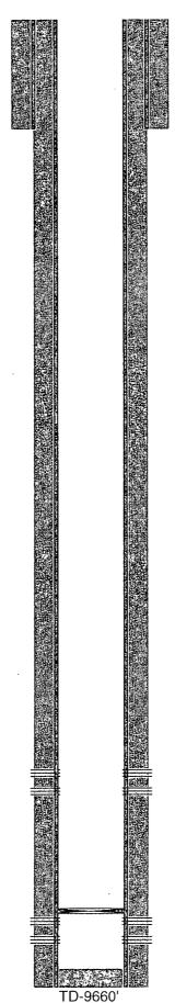
12-1/4" hole @ 1210' 9-5/8" csg @ 1210' w/ 875sx-TOC-Surf-Circ
