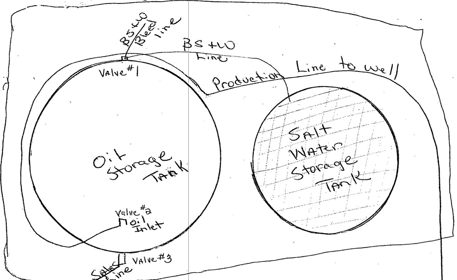
Valve #1 - Sealed close unless water needs bled off
