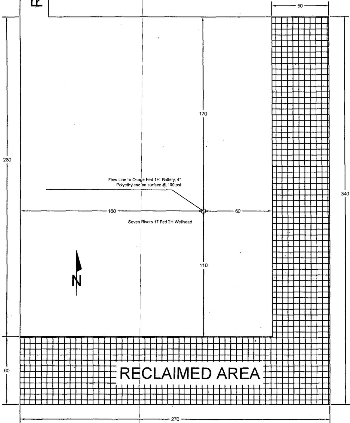
Flow Line to Osage Fed 1H Battery, 4" Polyethylene on surface @ 100 psi
