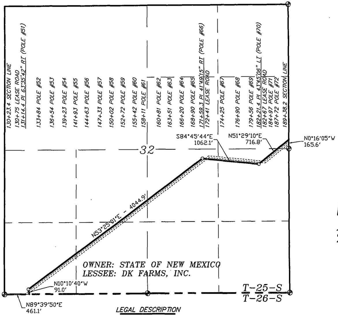
A STRIP OF LAND 30.0 FEET WIDE, LOCATED IN SECTION 32, TOWNSHIP 25 SOUTH, RANGE 31 EAST, N.M.P.M., EDDY COUNTY, NEW MEXICO AND BEING 15.0 FEET LEFT AND RIGHT OF THE FOLLOWING CENTERLINE SURVEY.
