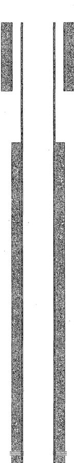
8-3/8" hole @ 369' 7" csg @ 369' w/ 50sx-TOC-Surf-Circ
