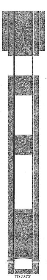
8-3/8" hole @ 369' 7" csg @ 369' w/ 50sx-TOC-Surf-Circ
