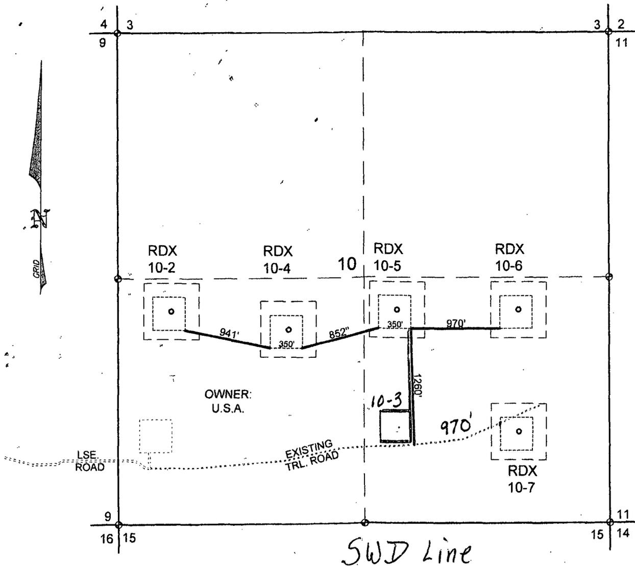
PROPOSED LEASE ROADS BEING 4023 FEET, 0.76 MILE OR 243.82 RODS IN LENGTH, SITUATED IN SECTION 10, TOWNSHIP 26 SOUTH, RANGE 30 EAST, N.M.P.M., EDDY COUNTY, NEW MEXICO, AND BEING 15 FEET LEFT AND 15 FEET RIGHT OF THE SURVEY OF CENTERLINE AS SHOWN HEREON.
