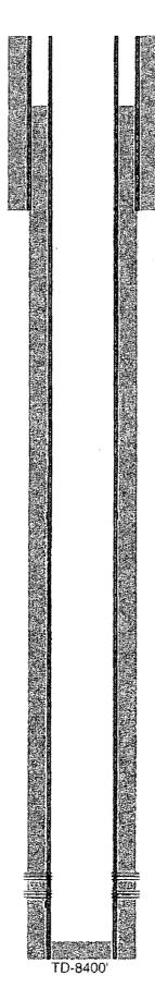
12-1/4" hole @ 1602' 9-5/8" csg @ 1602' w/ 800sx-TOC-Surf-Circ
