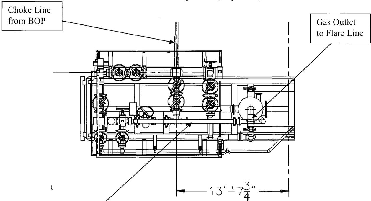
**Choke Manifold – Gas Separator (Side View)**
