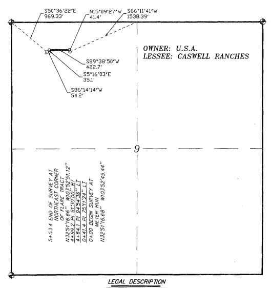
A STRIP OF LAND 30.0 FEET WIDE, LOCATED IN SECTION 9, TOWNSHIP 17 SOUTH, RANGE 31 EAST, N.M.P.M., EDDY COUNTY, NEW MEXICO AND BEING 15.0 FEET LEFT AND RIGHT OF THE ABOVE PLATTED CENTERLINE SURVEY.
