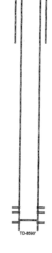
17-1/2" hole @ 371' 13-3/8" csg @ 371' w/ 950sx-TOC-Surf-Circ (1")
