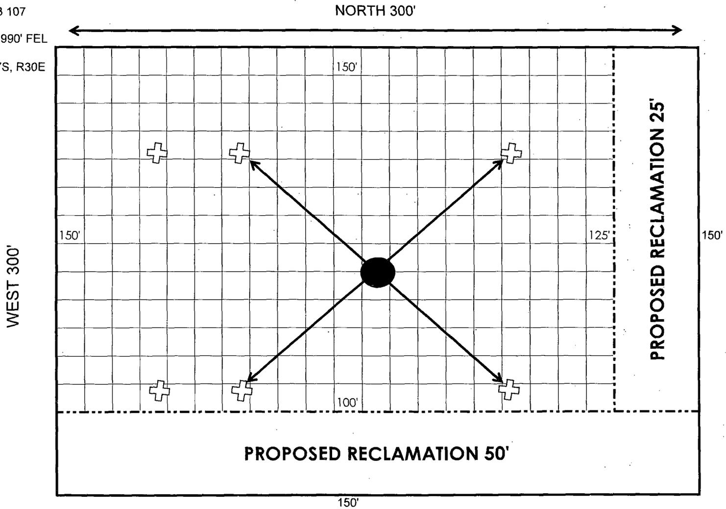
✚ ANCHOR 75' FROM WELLHEAD TO ANCHORS
