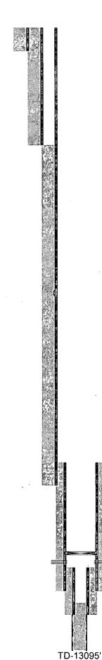
26" hole @ 606' 20" csg @ 606' w/ 1330sx-TOC-Surf-Circ
