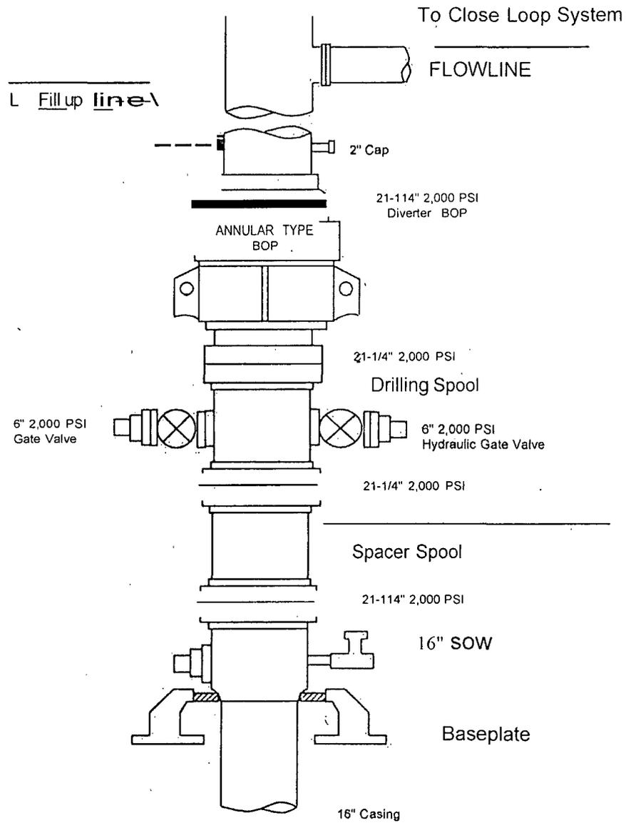
**Diverter system will be rigged up to the Choke Manifold Diagrams provided.**
