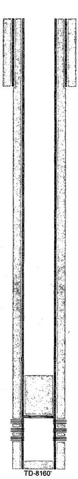
12-1/4" hole @ 1208' 9-5/8" csg @ 1208' w/ 880sx-TOC-Surf-Circ
