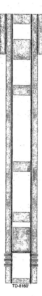
12-1/4" hole @ 1208' 9-5/8" csg @ 1208' w/ 880sx-TOC-Surf-Circ
