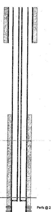
8-1/2" hole @ 464' 7" csg @ 464' w/ 100sx-TOC-Surf-Circ
