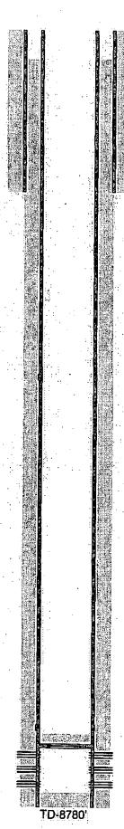
12-1/4" hole @ 1825' 9-5/8" csg @ 1820' w/ 993sx-TOC-Surf-Circ
