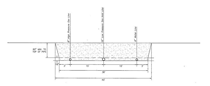
BACKFILL DIRT TO BE AS FREE OF ROCKS AND LARGE PARTICLES AS POSSIBLE
