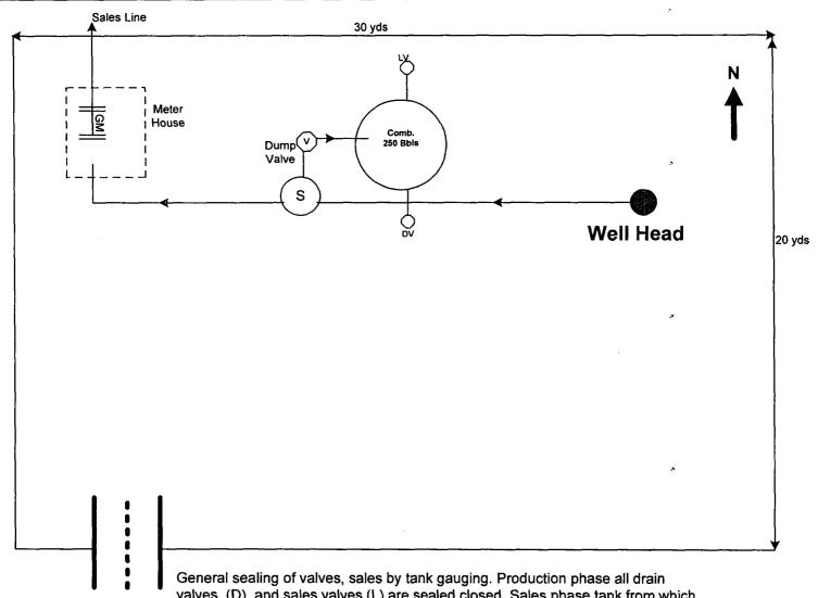
valves, (D), and sales valves (L) are sealed closed. Sales phase tank from which sales are made is isolated by sealing closed the drain, fill and equalizer valves during sales. Draining phase the tank being drained will be isolated by sealing closed the sales, fill and equalizer valve. The drain valve on the other tank will be sealed closed.
