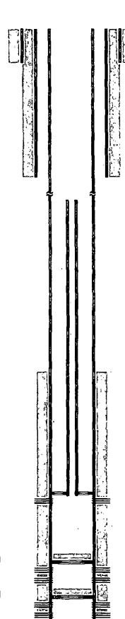
17-1/2" hole @ 620' 13-3/8" csg @ 620' w/ 700sx-TOC-Surf-Circ
