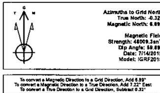
To convert a Magnetic Direction to a Grid Direction, Add 0.89°
