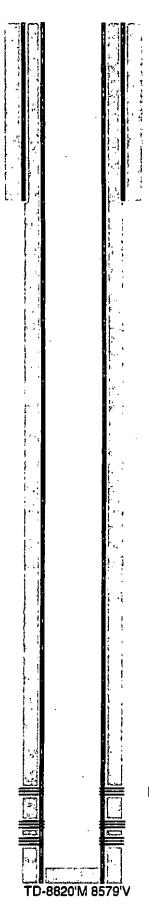
12-1/4" hole @ 1825' 9-5/8" csg @ 1825' w/ 1375sx-TOC-Surf-Circ
