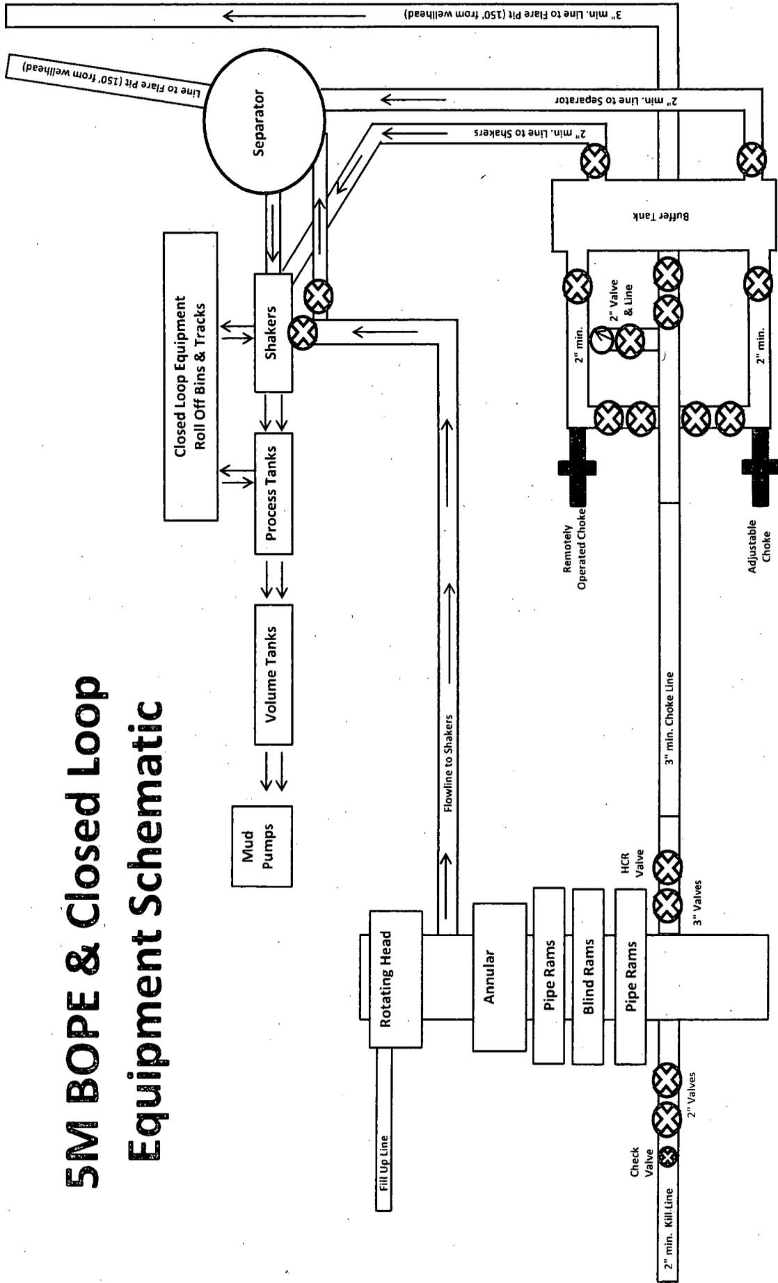
Note: All valves & lines on choke manifold are 3" unless otherwise noted. Exact manifold configuration may vary.
