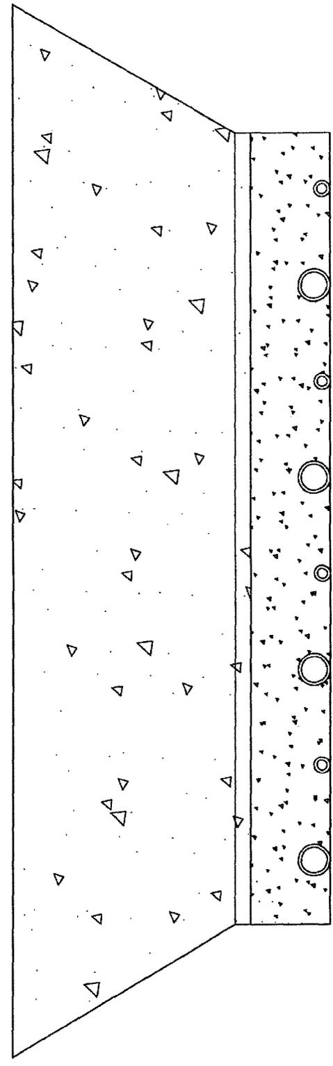
BACKFILL DIRT TO BE AS FREE OF ROCKS AND LARGE PARTICLES AS POSSIBLE
