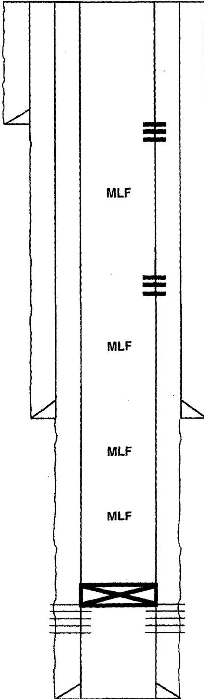
Perf at 490' and squeeze 120sx of Class "C" cement from 490'-surface.
