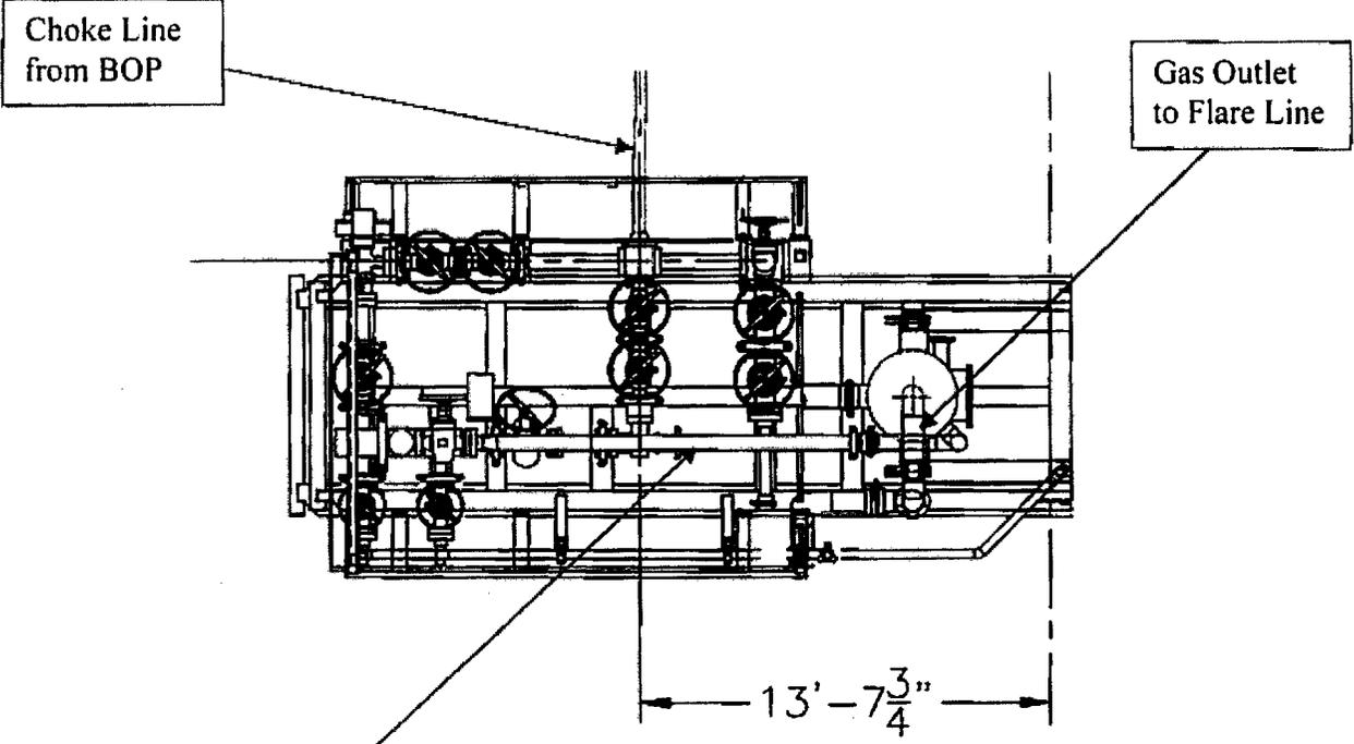
**Choke Manifold – Gas Separator (Side View)**
