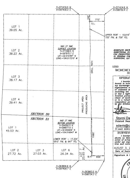
BOREPATH SHOWN HEREON IS BASED ON DIRECTIONAL SURVEY REPORT PROVIDED BY COG PRODUCTION LLC FOR THE COPPERHEAD 31 FEDERAL COM 39H SUPPLIED TO HARCROW SURVEYING, LLC ON DECEMBER 20, 2016
