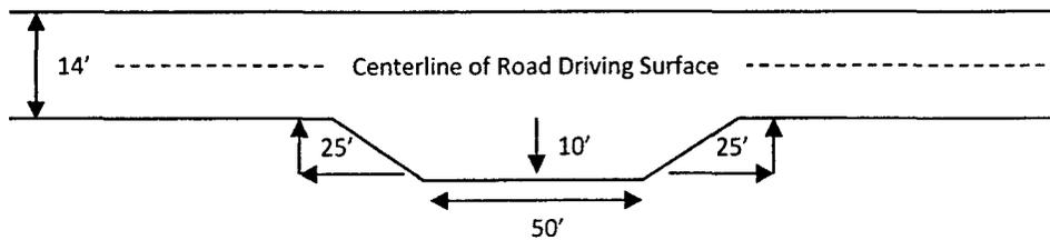
23. Drainage control systems shall be constructed on the entire length of road (e.g. ditches, sidehill outsloping and insloping, lead-off ditches, culvert installation, and low water crossings).
