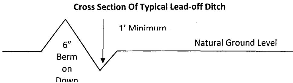
25. All lead-off ditches shall be graded to drain water with a 1 percent minimum to 3 percent maximum ditch slope. The spacing interval are variable for lead-off ditches and shall be determined according to the formula for spacing intervals of lead-off ditches, but may be amended depending upon existing soil types and centerline road slope (in %);
