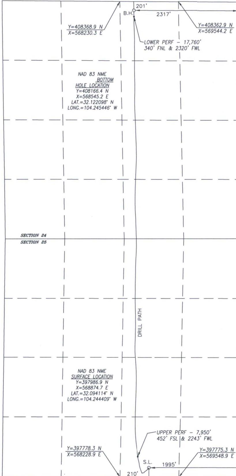
BOREPATH SHOWN HEREON IS BASED ON DIRECTIONAL SURVEY REPORT PROVIDED BY COG FOR THE ROAD RUNNER FEDERAL COM #12H SUPPLIED TO HARCROW SURVEYING, LLC ON 12/22/17.
