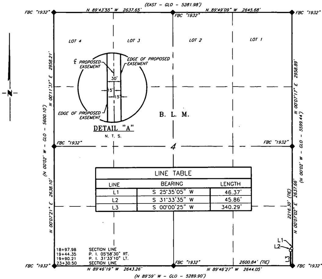
A strip of land 30 feet wide, being 432.52 feet or 26.213 rods in length, lying in Section 4, Township 22 South, Range 23 East, N. M. P. M., Eddy County, New Mexico, being 15 feet left and 15 feet right of the following described survey of a centerline across B. L. M. land:
