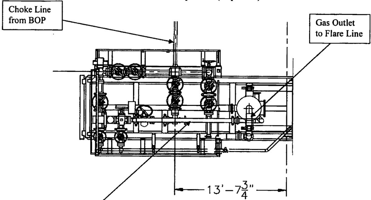
**Choke Manifold – Gas Separator (Side View)**
