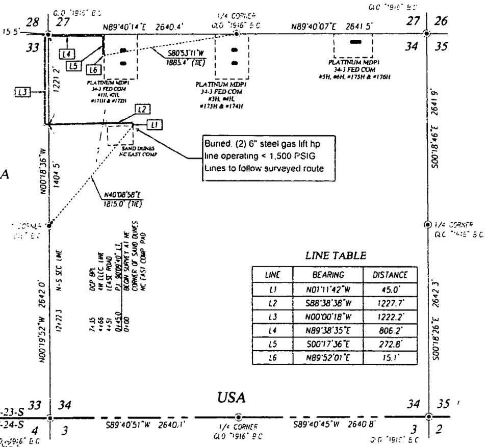
Buried (2) 6" steel gas lift hp line operating < 1,500 PSIG
