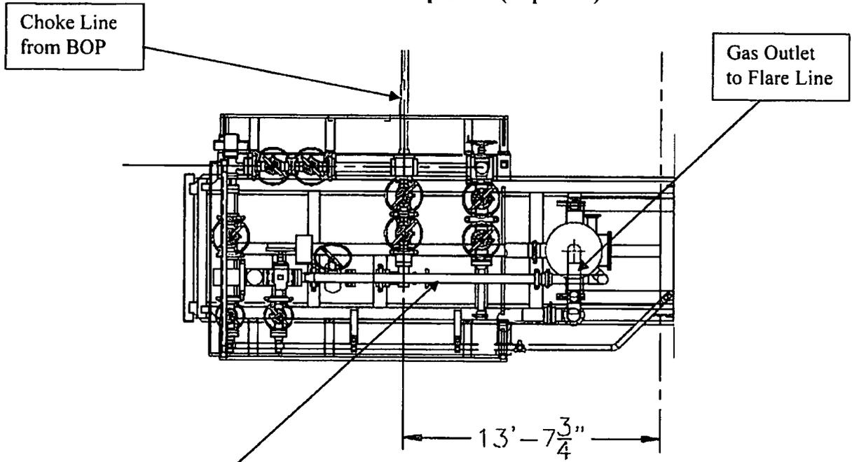
**Choke Manifold – Gas Separator (Side View)**
