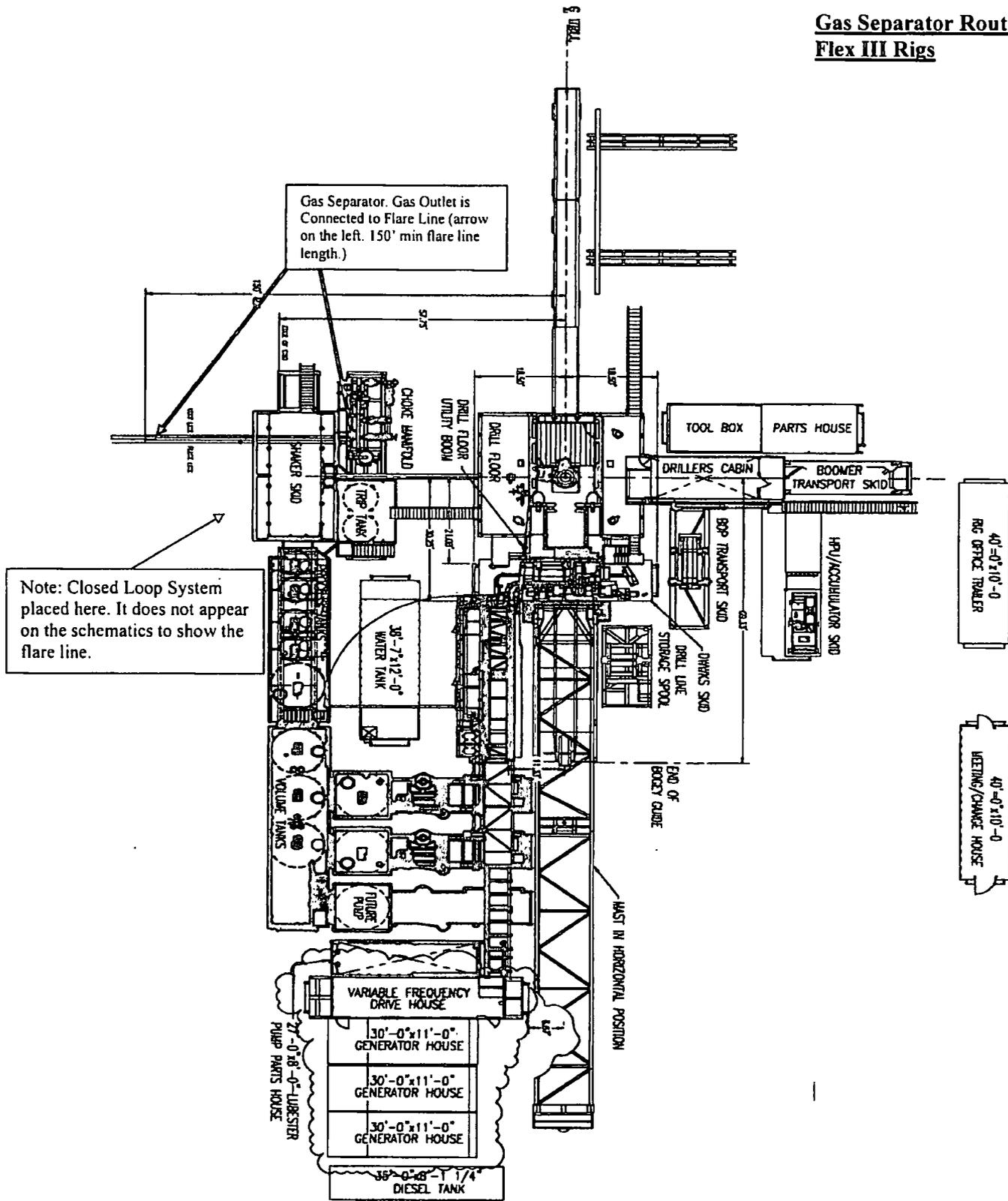
**Choke Manifold – Gas Separator (Top View)**
