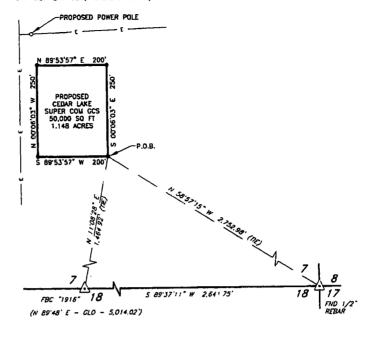
NOTE: CENTER OF GAS COMPRESSOR STATION IS LOCATED AT 1561' FSL & 2450' FEL
