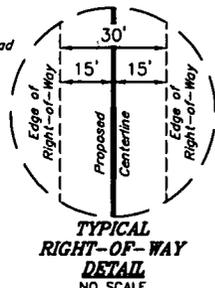
BEGINNING OF PROPOSED GAS PIPELINE RIGHT-OF-WAY (At Edge of Pad)
