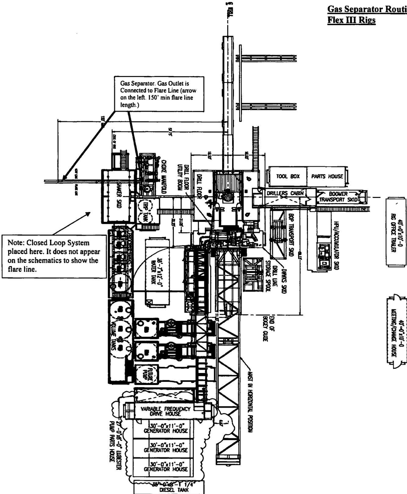
**Choke Manifold – Gas Separator (Top View)**
