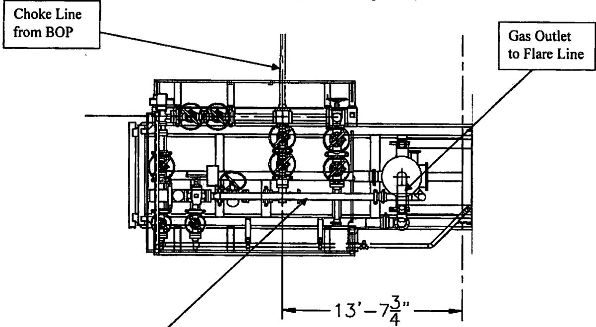
**Choke Manifold – Gas Separator (Side View)**
