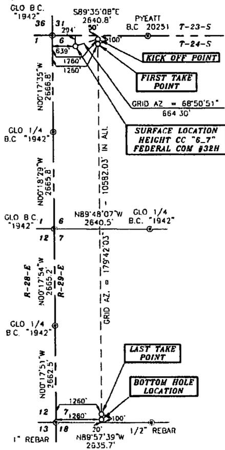
Data of Bearings - GPS Geodetic Measurements
