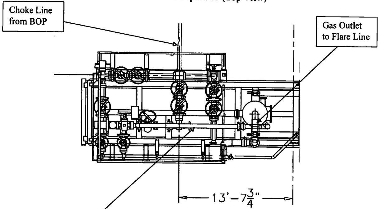
**Choke Manifold – Gas Separator (Side View)**
