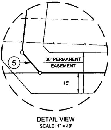
Being a proposed gasline easement being 30 feet in width, 15 feet left, and 15 feet right of the above platted centerline total line footage containing 3446.98 feet or 208.91 rods, containing 2.37 acres more or less.
