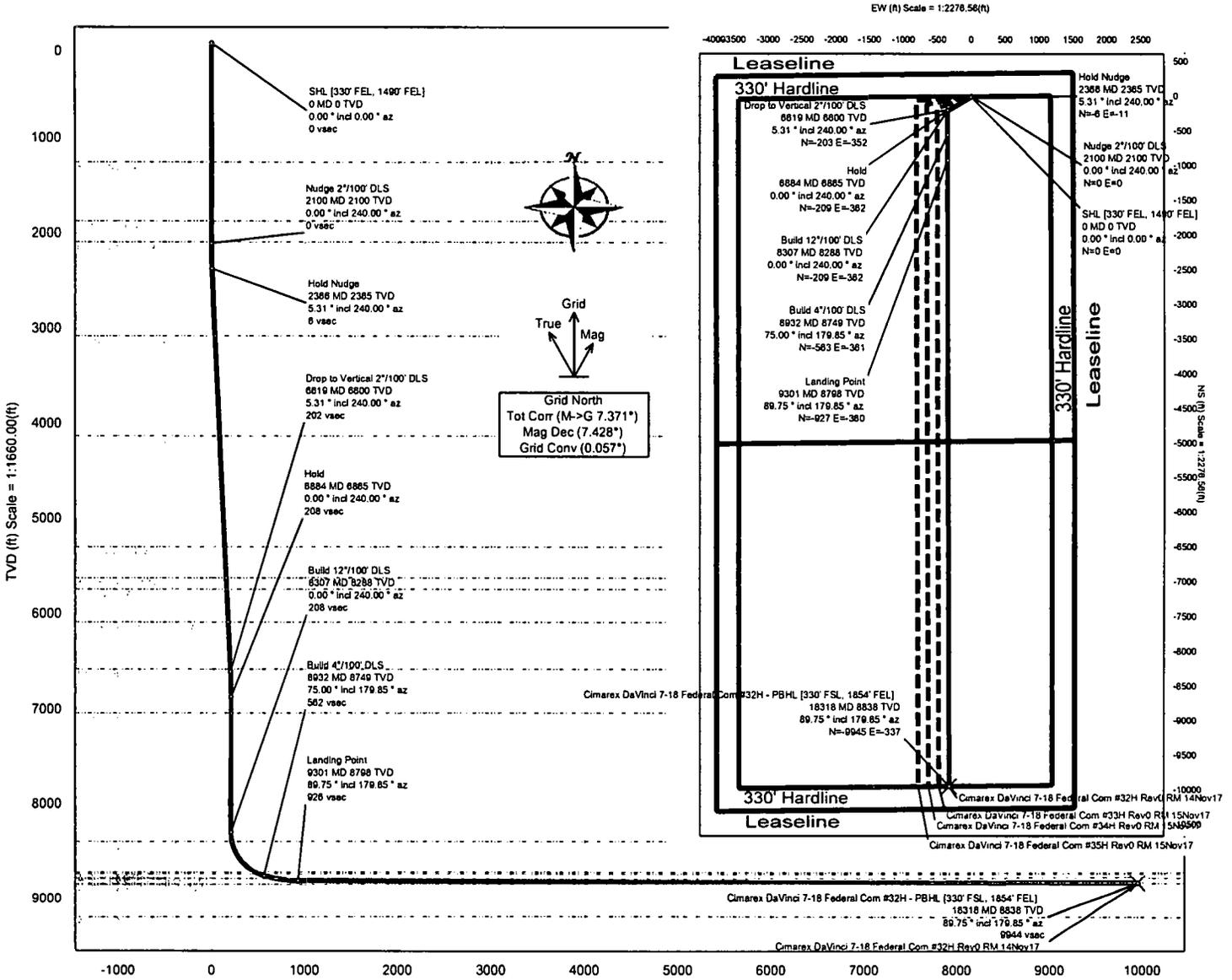
Vertical Section (ft) Azim = 179.85° Scale = 1:1660.00(ft) Origin = 0N/-S, 0E/-W
