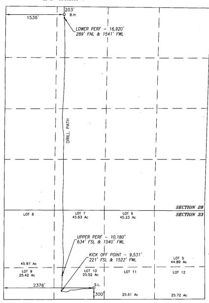
NAD 83 NME SURFACE LOCATION Y=364249.3 N X=647601.2 E LAT.=32.000938\* N LONG.=103.990531° W BOREPATH SHOWN HEREON IS BASED ON DIRECTIONAL SURVEY REPORT PROVIDED BY COG OPERATING, LLC FOR THE LITTLEFIELD 33 FEDERAL COM #706H SUPPLIED TO HARCROW SURVEYING, LLC ON MAY 23, 2019
