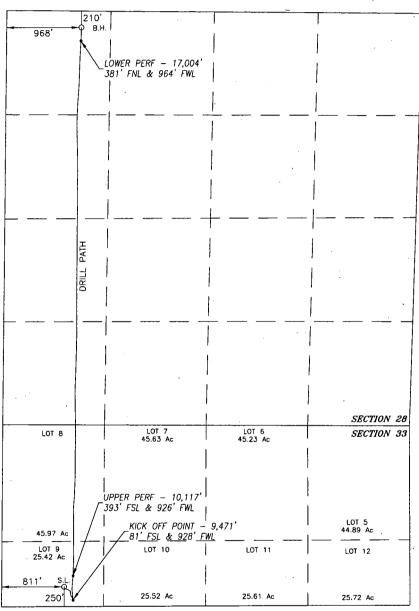
NAD 83 NME <u>SURFACE LOCATION</u> Y=364195.2 N X=646036.3 E LAT.=32.000803\* N LONG.=103.995580\* W BOREPATH SHOWN HEREON IS BASED ON DIRECTIONAL SURVEY REPORT PROVIDED BY COG OPERATING, LLC FOR THE LITTLEFIELD 33 FEDERAL COM #707H SUPPLIED TO HARCROW SURVEYING, LLC ON MAY 23, 2019
