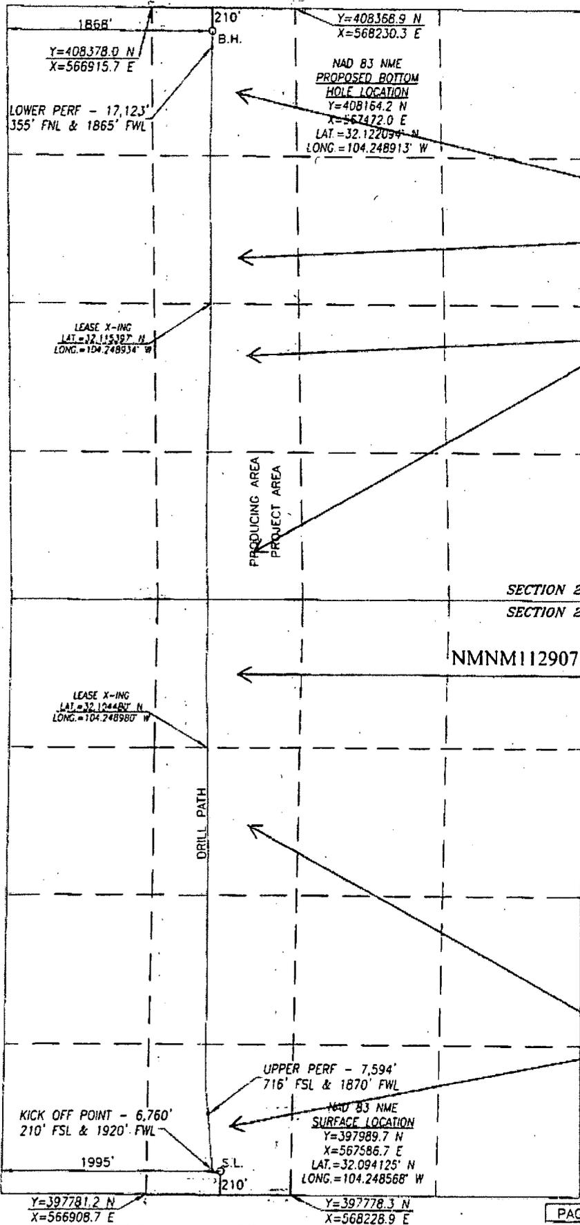
BOREPATH SHOWN HEREON IS BASED ON DIRECTIONAL SURVEY REPORT PROVIDED BY COG OPERATING, LLC FOR THE ROADRUNNER FEDERAL COM #3H SUPPLIED TO HARCROW SURVEYING, LLC ON NOVEMBER 7, 2018
