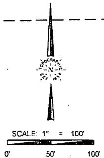
ALL BEARINGS, DISTANCES, AND COORDINATE VALUES CONTAINED HEREON ARE GRID BASED UPON THE NEW MEXICO COORDINATE SYSTEM OF 1983, EAST ZONE, U.S. SURVEY FEET
