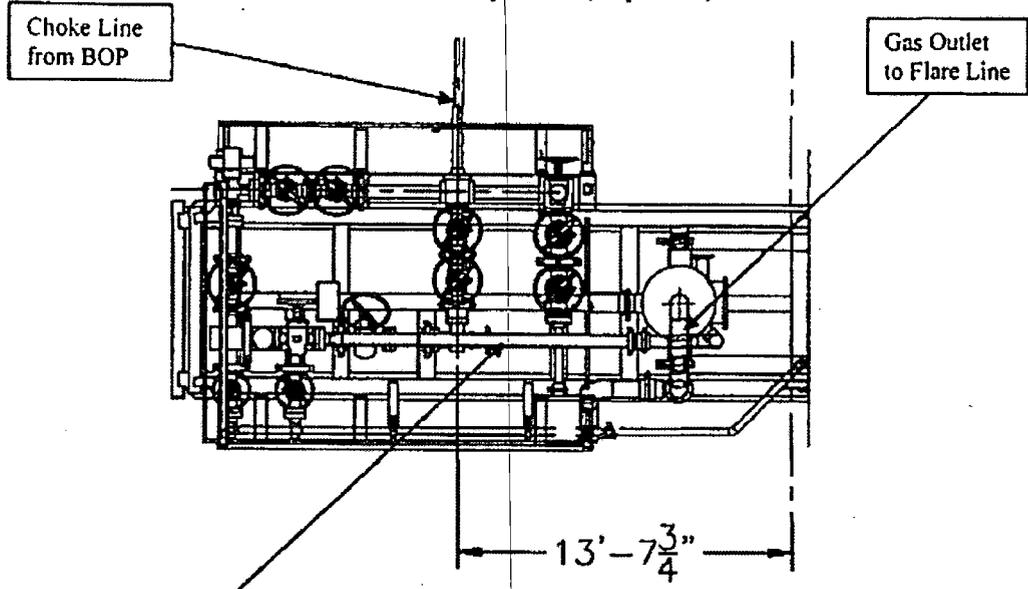
Choke Manifold – Gas Separator (Side View)
