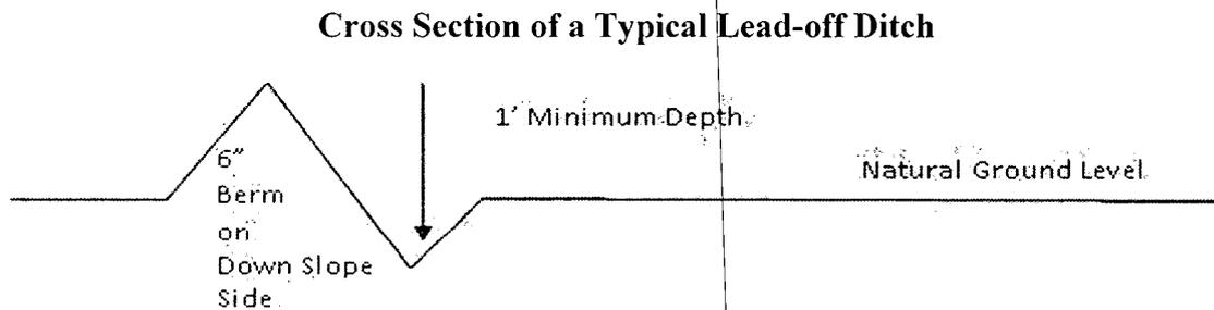
All lead-off ditches shall be graded to drain water with a 1 percent minimum to 3 percent maximum ditch slope. The spacing interval are variable for lead-off ditches and shall be determined according to the formula for spacing intervals of lead-off ditches, but may be amended depending upon existing soil types and centerline road slope (in %);
