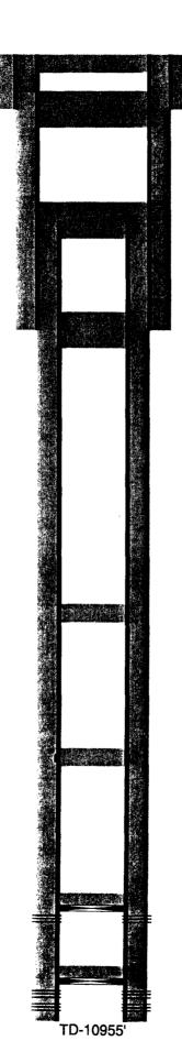
17-1/2" hole @ 475' 13-3/8" csg @ 475' w/500sx-TOC-Surf-Circ
