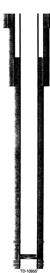
17-1/2" hole @ 475' 13-3/8" csg @ 475' w/500sx-TOC-Surf-Circ
